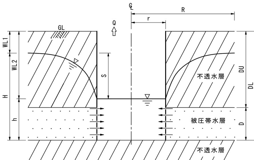
$$Q = \frac{2 \times \pi \times K \div 100 \times D \times (H - h)}{\ln(R \div r)} \times 60$$
