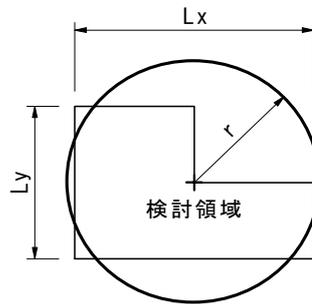
$$r1 = \sqrt{(Lx \times Ly \div \pi)} \quad \dots \quad \text{等価面積円}$$
